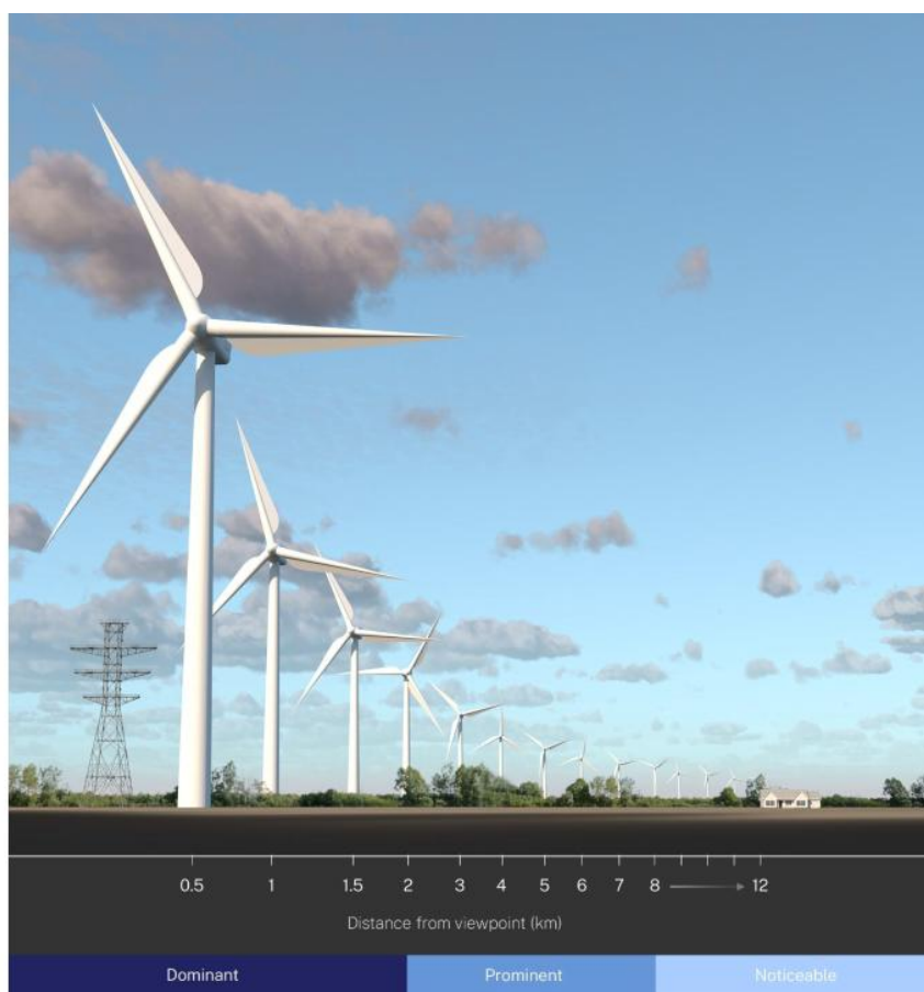
Figure 1 - Visual prominence of 250m turbines at varying distances (NSW Department of Planning, Housing and Infrastructure, Wind Energy Guideline).
